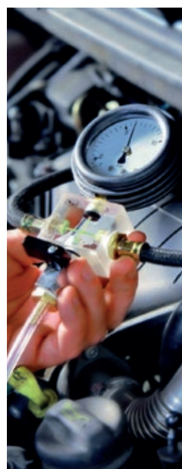
CR INJECTOR RETURN FLOW PRESSURE
