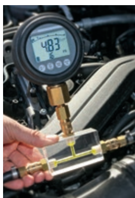
FUEL LOW PRESSURE MEASUREMENT AND AIR BUBBLE FREE
