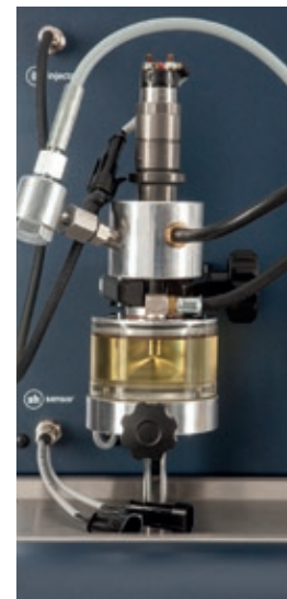
TEST STANDS FOR CR AND GDI INJECTORS, WITH TEST CERTIFICATE
